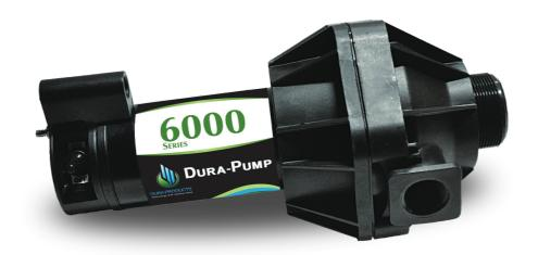
The DURA-PUMP™ 6000 Series (DP-6000) Transfer Pump is a 12 Volt DC or 110 Volt AC, non-UL rated, self-priming, positive-displacement diaphragm pump. It is designed for non-flammable fluid transfer and recirculation. The pump includes a 20' power cord with alligator clips and an inline fuse. The pump features a 1-inch NPT inlet and a 1-inch NPT discharge port.
